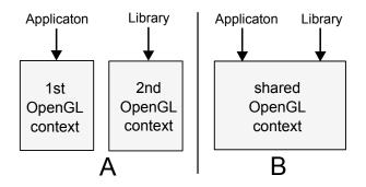
Figure 2: A - two separate OpenGL contexts, B - single shared OpenGL context
